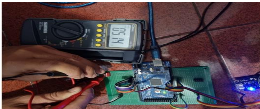
Gambar 6. Pengujian Power Supply
