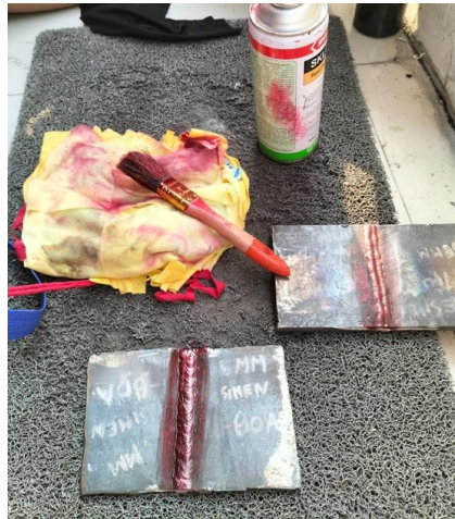
Gambar 4: Proses Pengujian Non Destructive Test
