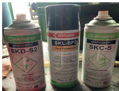
Gambar 3: Remover (SKC-S), Penetrant (SKL-SP2), Developer (SKD-S2).
