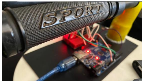
Gambar 4.1 Antilock Brake System & Auto Brake System for Motorcycle (Prototipe) Antilock Brake System & Auto Brake System for Motorcycle (Prototipe).
